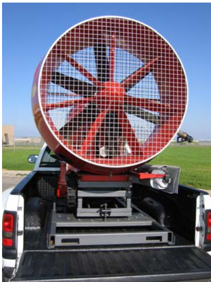
Skid Frame mounted in truck bed
